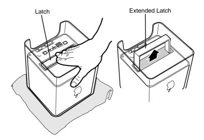
Allow the latch to extend completely.
